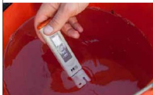
FIGURE 3.10 Checking the pH level in water using a digital meter
